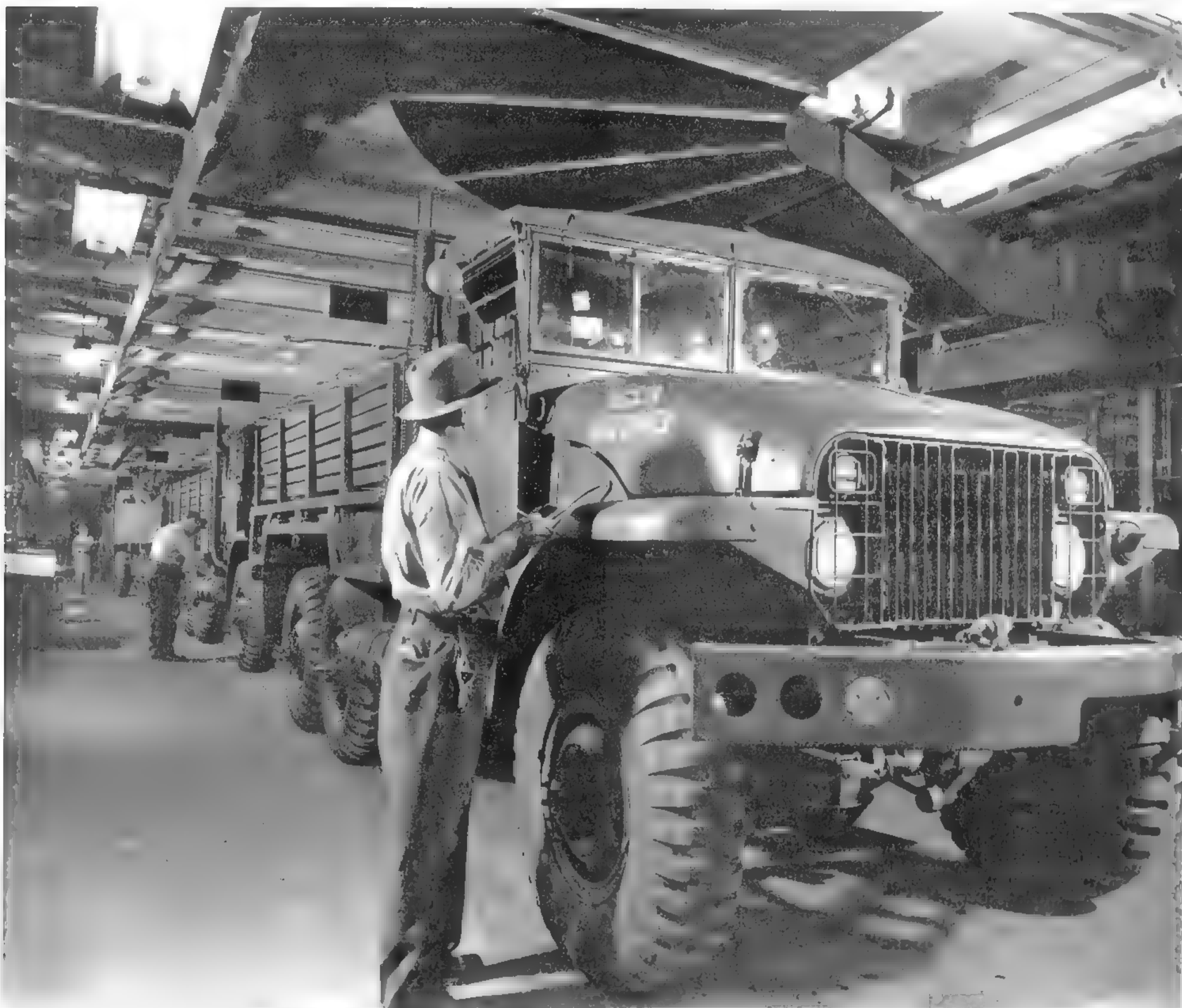
This M135 cargo truck was photographed just after final inspection at the GMC Yellow Truck and Coach plant. The characteristic holed front bumper is visible, as is the vertical exhaust stack. (GMC Truck and Coach photo)
